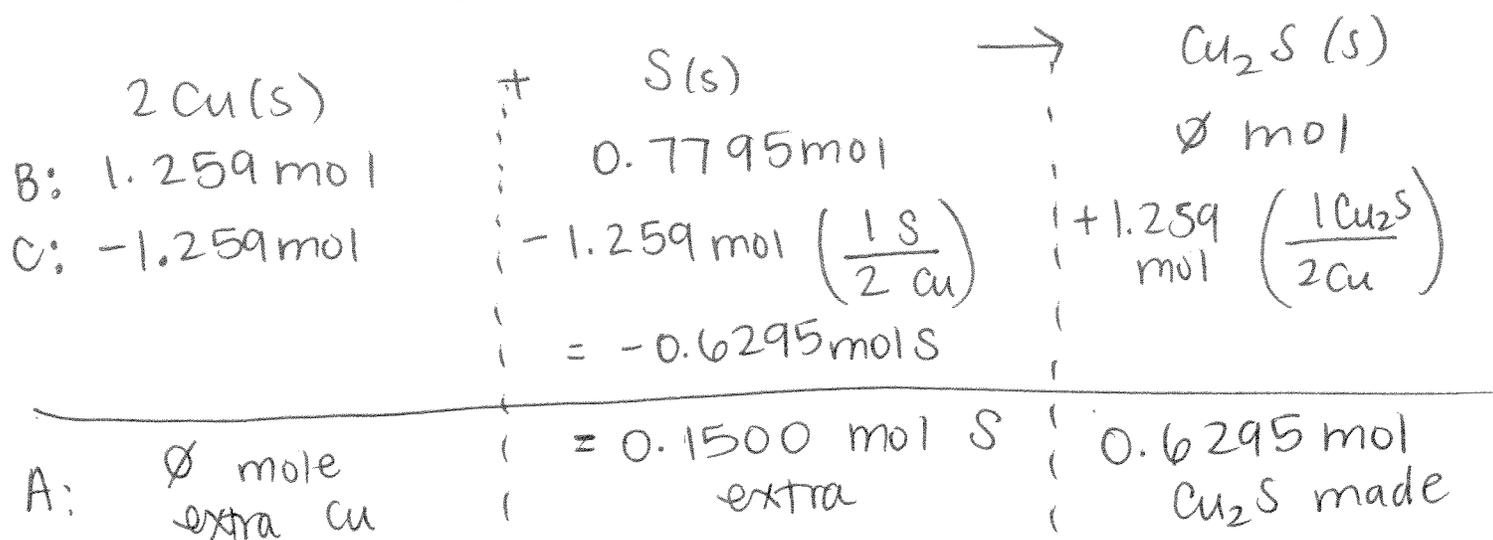
$$\text{a) } \frac{0.6295\text{ mol Cu}_2\text{S}}{1\text{ mol Cu}_2\text{S}} \left| \frac{159.17\text{g Cu}_2\text{S}}{1\text{ mol Cu}_2\text{S}} \right. = \boxed{100.2\text{g Cu}_2\text{S}}$$
